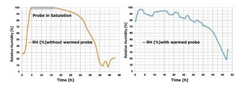
A 48-hour drying cycle with the old system (left) and the Vaisala HMT337 with warmed probe (right). The warmed-probe technology provides accurate relative-humidity readings at the beginning of the process, where the non-heated probe is saturated by condensed water.
