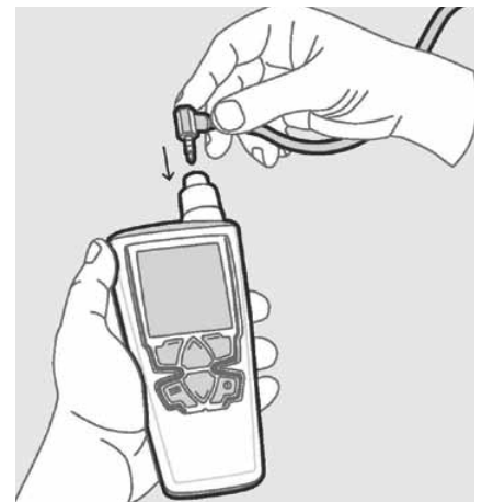
Snapping a connector to the indicator HM40 to read the measurement results.
