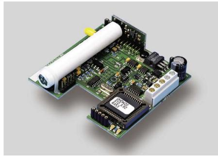
The Vaisala CARBOCAP<sup>®</sup> Carbon Dioxide Module GMM20W is designed for OEM applications in benign environments.
