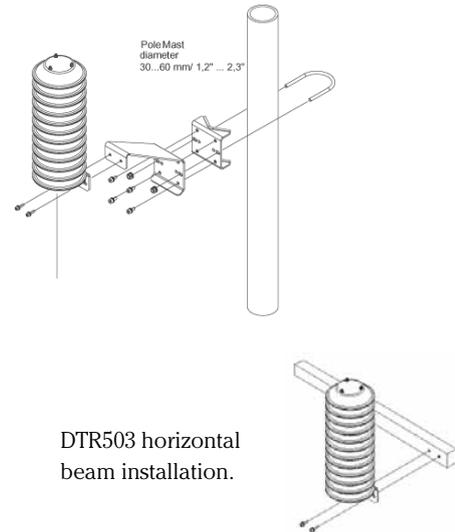
DTR503 horizontal beam installation.
