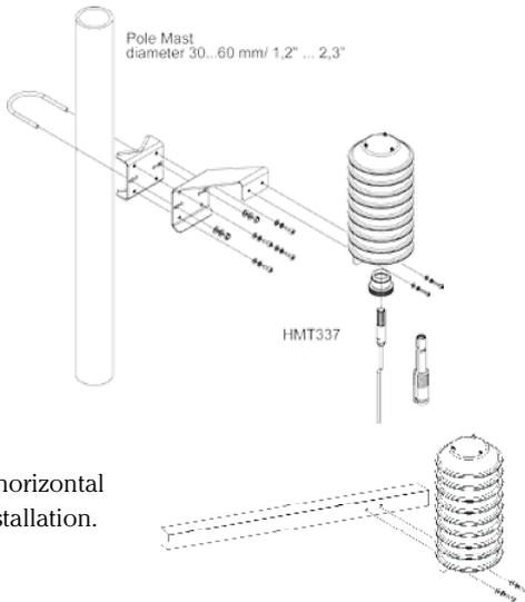
DTR502 horizontal beam installation.
