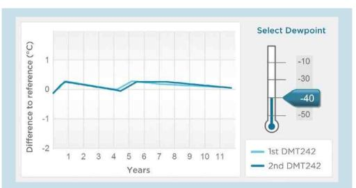
The graphs above are derived from an ongoing test in which two Vaisala DRYCAP® DMT242 dewpoint transmitters were installed in a compressed air line ca 11 years ago and have not been recalibrated or adjusted. The line conditions are representative of instrument air. The x-axis represents years, the y-axis represents difference to the reference value at periodic checks.
