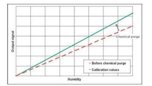
The purge function briefly heats the sensor in order to remove any volatile contaminants from the polymer.
